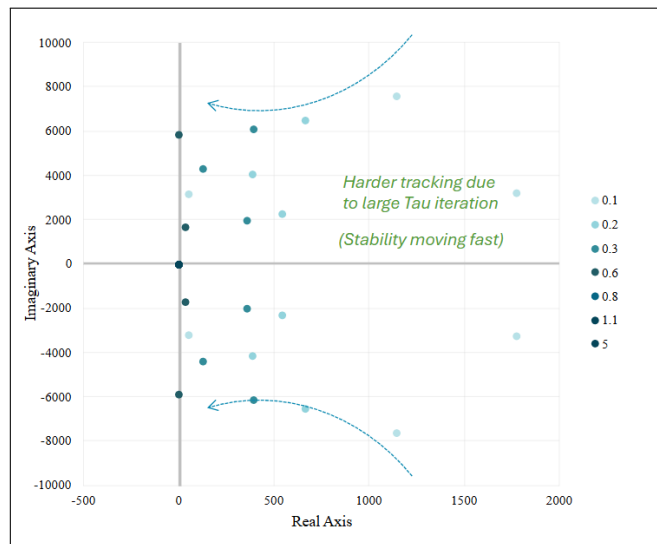
Figure 23: Eigenvalue plot showing the tuning of \tau_{pq} after adding one VSC
